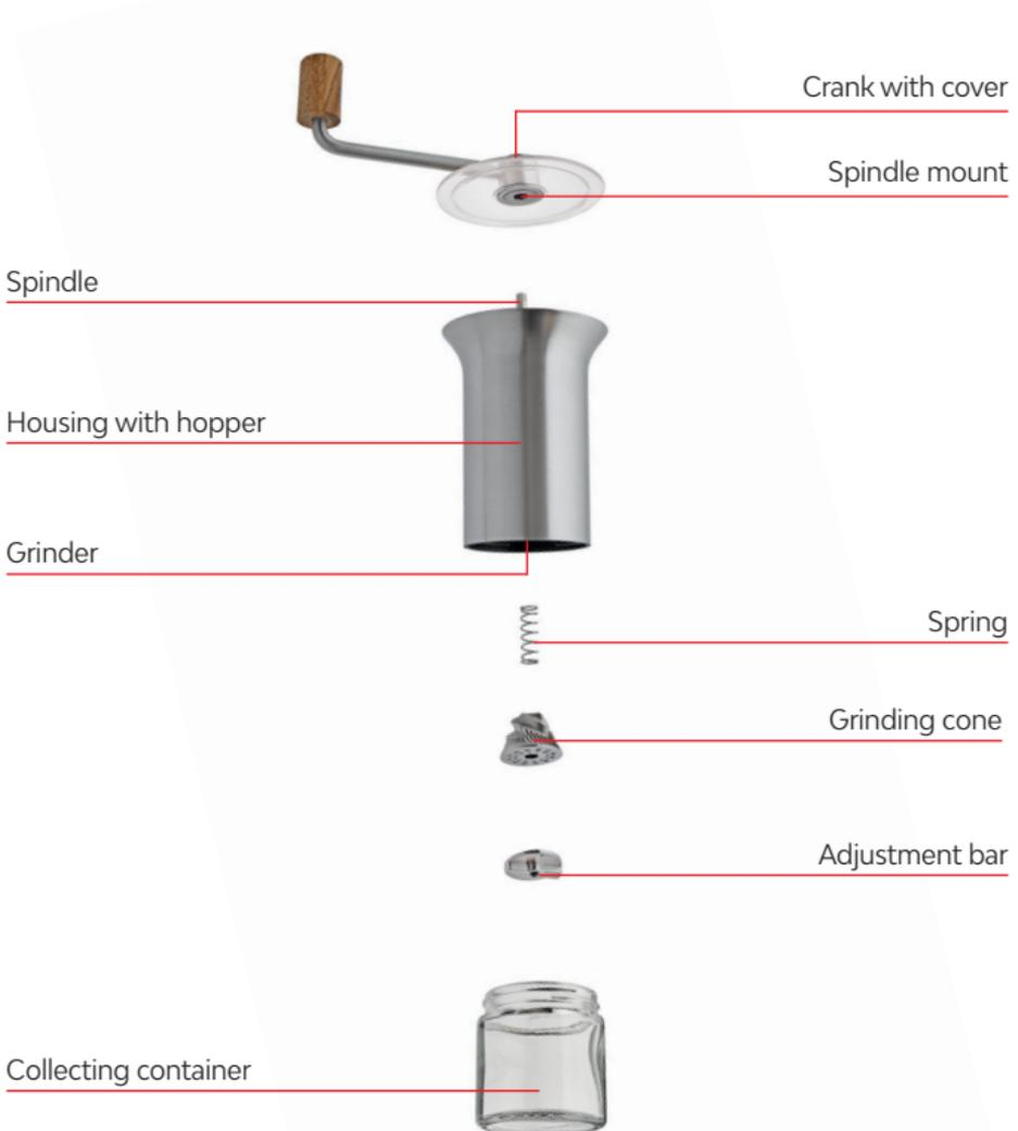
Unscrew the collecting container. Hold the crank with cover and turn the mill upside down. Turn the adjustment bar anti-clockwise until it releases from the grinder and take it off. Remove grinding cone and spring.
