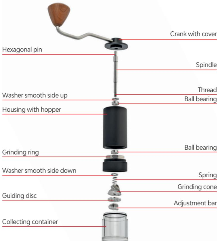
Remove the collecting container. Hold the crank with cover and turn the mill upside down. Turn the adjustment bar anti-clockwise until it releases from the grinder and take it off. Remove all grinder components. Unscrew the grinding ring clockwise.
